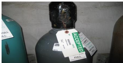
Figure 1. Gas Cylinder Example. The figure displays a compressed gas cylinder with CIDB inventory tag on suspended hang tag.
