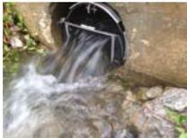
Fig. 1: Thelmar weir used at MC inlets, HR inlets and outlets.
