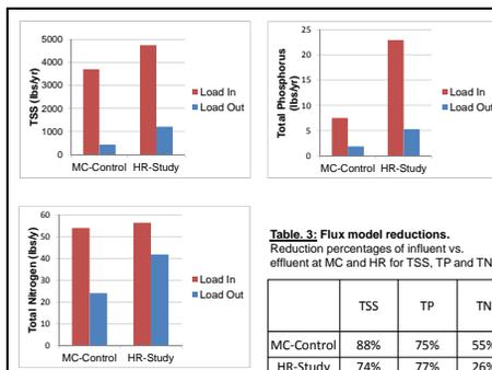
Fig. 4: Flux model results. Influent and effluent loads (lbs/yr) of pollutants at MC and HR for TSS, TP and TN.
