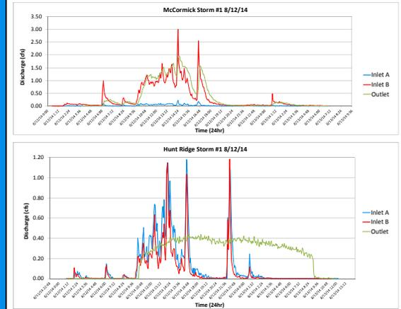
Fig. 4: Storm hydrographs were created to accurately determine rising limb, peak and falling limb times and volumes. Discharge amounts are highly dependent on preceding conditions: precipitation amount and intensity, drainage area and percent impervious.
