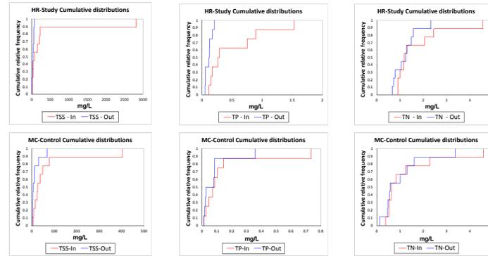
Fig. 3: Cumulative distribution plots of TSS, TP and TN at HR-Study and MC-Control facilities.
