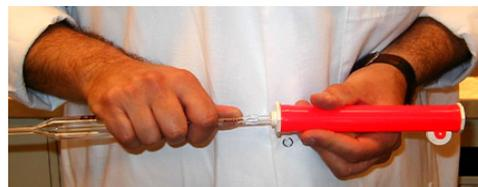
The 10 ml plastic pipettes have two scales on them that run in opposite directions. When measuring liquid, use the scale that has the “1 ml” at the bottom tip and “10 ml” at the top. Also, make sure to use the bottom of the meniscus (the curved part of the liquid in the pipette) to determine the volume level. When transferring liquid, make sure the container you are transferring the liquid into is nearby or liquid may start to drip out of the pipette tip. The transfer must take place quickly.
