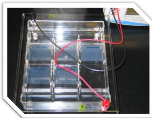
Figure 4. Gel box connected to power supply
