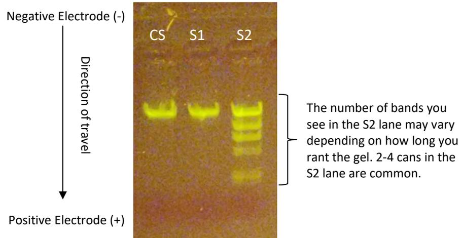
Figure 5. In this example, the sample from Suspect 1 (S1) matches the DNA found at the Crime Scene (CS). The DNA from Suspect 2 (S2) does not match the DNA found at the Crime Scene.
